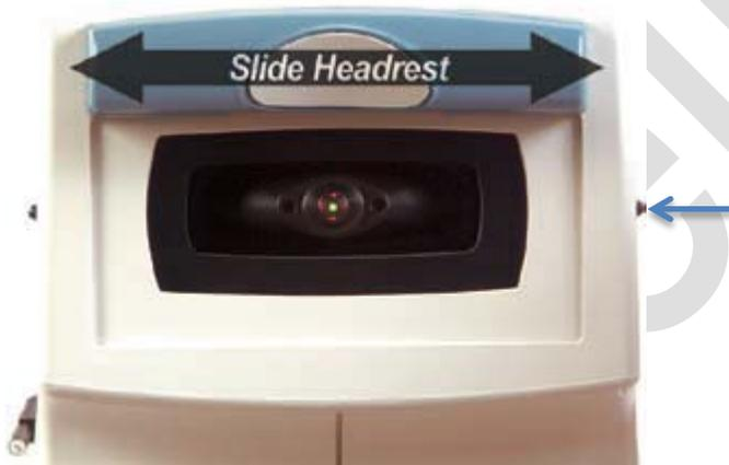
**Step 4:** Adjust the headrest to the right or left to enable the software to automatically determine which eye is being measured. The headrest must be positioned completely to one side or to the other in order to take a measurement. Start with the **right eye** by sliding the headrest to the participant's left.
